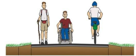
TRAIL THROUGH LIVINGSTON INDUSTRIAL COMPLEX 8' or 10' Wide Trail – Asphalt or Stone Dust
